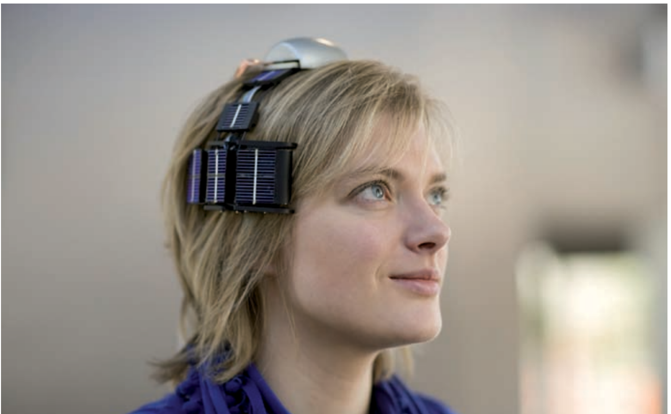
The wearable wireless EEG system with hybrid power supply.
