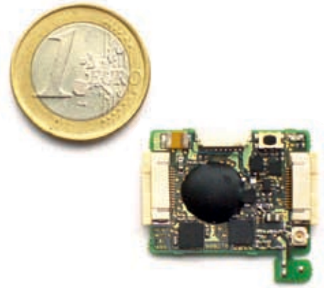
Wireless sensor platform.
