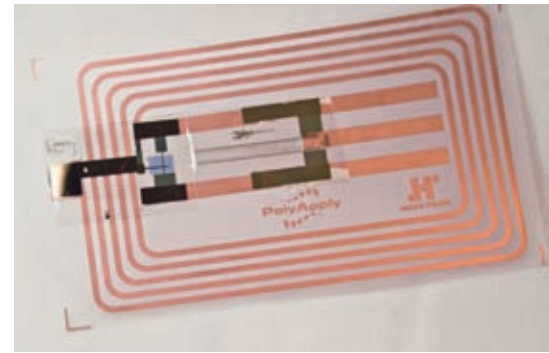
A fully flexible, 64-bit organic RFID tag generated by laminating the antenna foil, the organic rectifier foil and the 64-bit organic digital logic foil.
