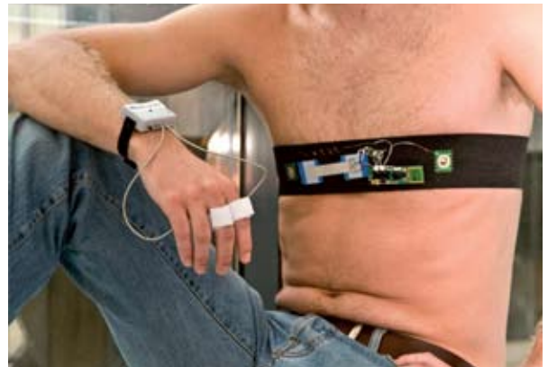
Wireless body area network for arousal monitoring: physiological signals are monitored, wirelessly transmitted and analyzed to extract, in real-time, the arousal level characteristic of a person's emotional state.
