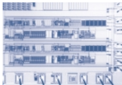
Layout of the analog port of the PDFE ASIC
