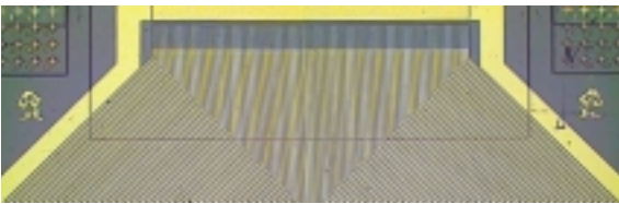
Extended-wavelength InGaAs linear detector array
