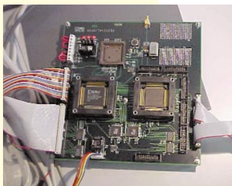
OFDM-modem development board.
