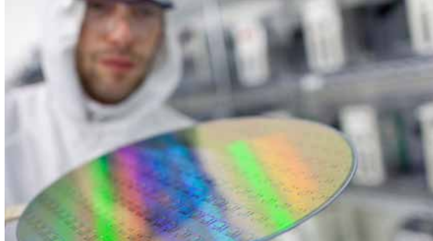
01 | 300mm silicon wafer with hundreds of chips.
